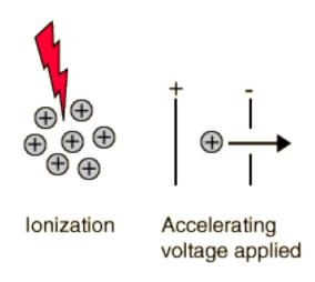
After ionization, acceleration, and selection of single velocity particles, the ions move into a mass spectrometer region where the radius of the path and thus the postion on the detector is a function of the mass.
