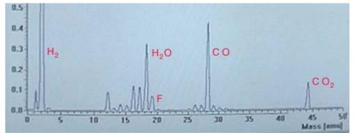
Residual gas analyzer mass spectrum of a UHV system
